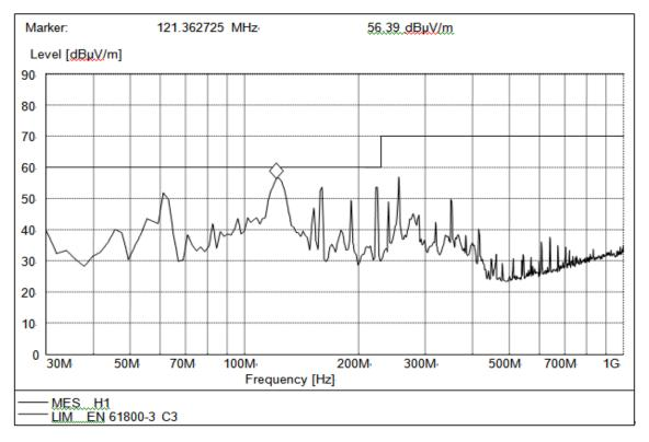
2. Electromagnetic radiation disturbances, max peak detector, antenna polarization: Vertical
